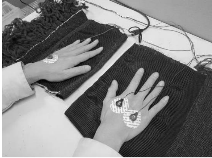
Fig. 2.4 The electrodes put anode on the left hand and cathod/GND on the right hand.
