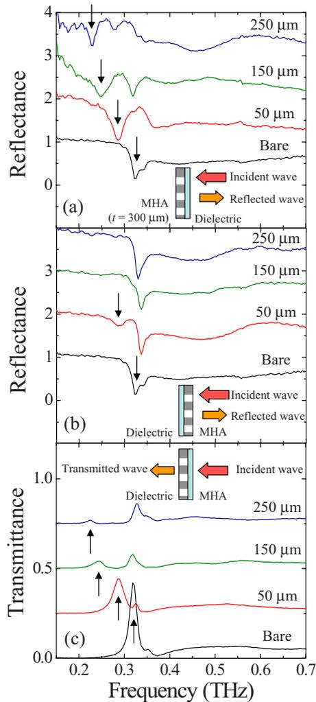
FIG. 2. (Color online) Measured reflection spectra for the 300  $\mu\text{m}$  thick MHA with PP films of several thicknesses  $t_{\text{PP}}$  attached to the (a) illuminated and (b) opposite sides of the array. (c) Measured transmission spectra for the same sample as (a). Schematic pictures of the optical configuration are shown in each figure.
