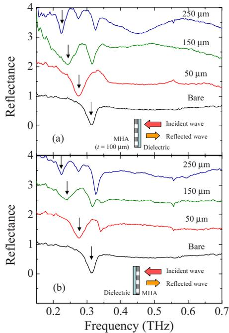
FIG. 3. (Color online) Measured reflection spectra for the 100  $\mu\text{m}$  thick MHA with PP films of several thicknesses  $t_{\text{PP}}$  attached to the (a) illuminated and (b) opposite sides of the array. Schematic pictures of the optical configuration are shown in each figure.
