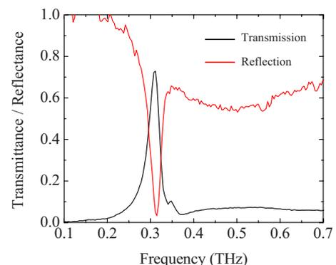
FIG. 1. (Color online) Measured reflection (red line) and transmission (black line) spectra for the 100  $\mu\text{m}$  thick MHA.
