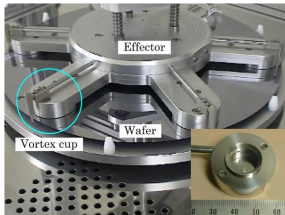
Fig. 2 Non-contact handling system by using swirling flow
