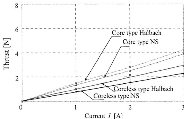
Fig. 10 Current-Thrust characteristic of a NS magnet array and a Halbach magnet array (measured).
