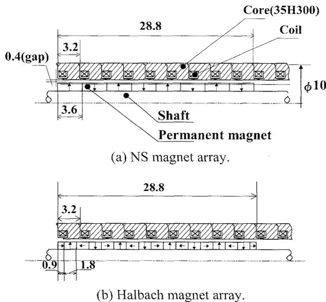
Fig. 2 Sectional structure of PCLM [units :mm].
