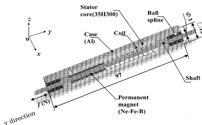
Fig. 1 Schematic structure of PCLM [units:mm].
