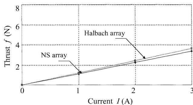
Fig. 8 Calculated thrust curves of coreless type.
