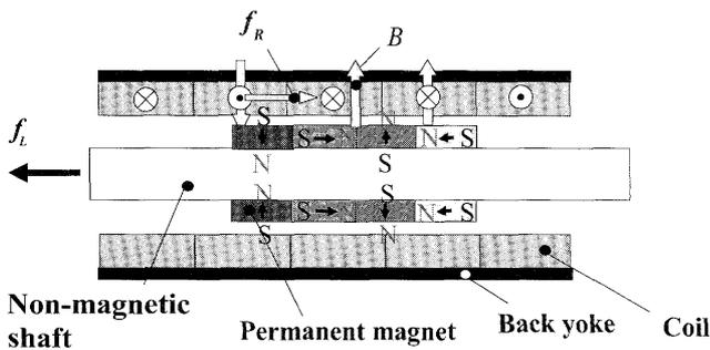
Fig. 3 Principle of operation.
