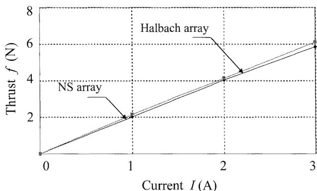
Fig. 7 Calculated thrust curves for the core type.
