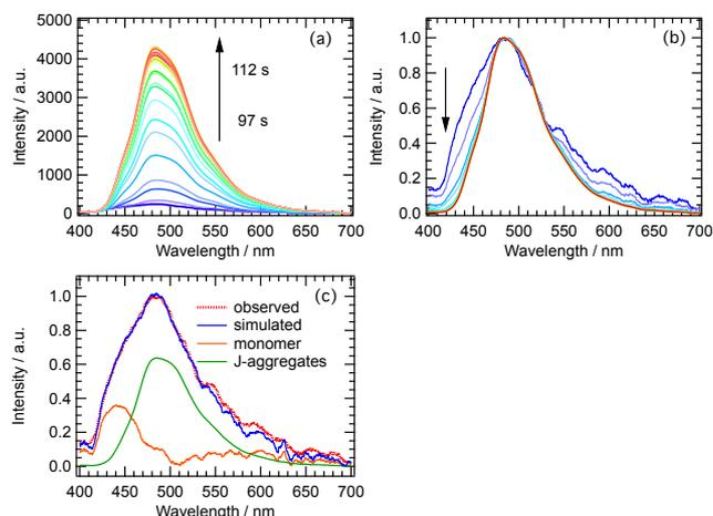
**Fig. 3** Fluorescence spectral changes (a) and normalized spectra (b) of  $5.0 \times 10^{-3} \text{ mol} \cdot \text{dm}^{-3}$  CN-MBE in a DCE droplet during solvent evaporation as a function of time. (c) The observed spectra after 97 s and simulated spectra from summation of the relative abundance of the planar conformational monomer and the J-aggregates by least-square fitting.
