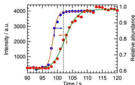
**Fig. 4** Change of fluorescence intensity (red circles) and relative abundance of J-aggregate (blue circles) of CN-MBE as a function of time. The solid line is a curve fit based on the sigmoidal function (see main text).
