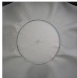
Figure 9. Wrinkling in the spherical crown.
