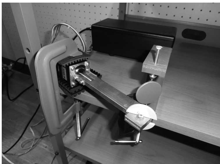
Figure 1 A photo of experimental devices for rotating (behind) and holding (front) hands. The disk on the device for holding hand is rotated by stepping motor, and the stepping motor is controlled by a function generator (which is not shown in this figure). The device for rotating hand is the same as used in Imai et al. (2018).
