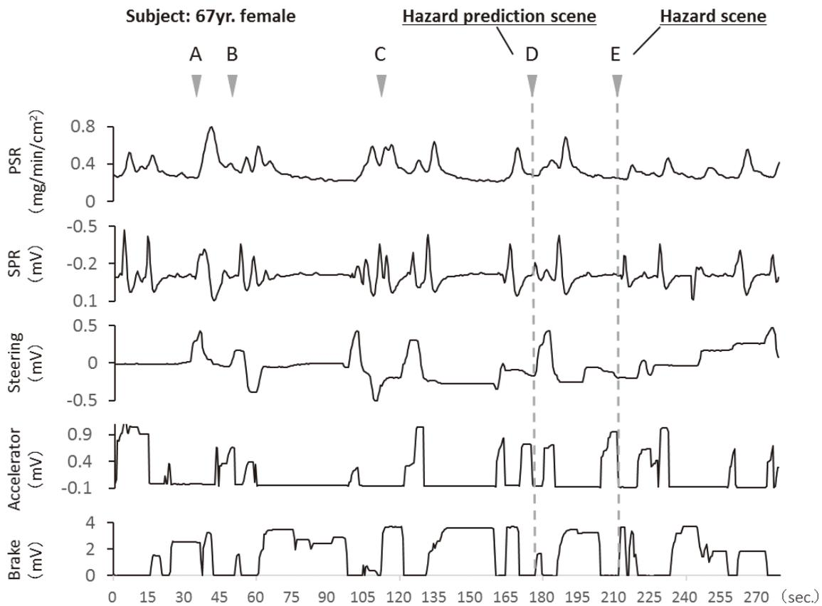
**Fig. 3.** Changes in PSR, SPR, and Reaction Volume of Steering Wheel, Accelerator, and Brake During Driving Simulation Test. [A] Jogger approaches from the opposite direction; [B] Vehicle approaches from the opposite direction; [C] Participant’s vehicle overtakes a bicycle; [D] Participant’s vehicle turns left at T-junction (hazard prediction scene); [E] Pedestrian runs out from a side street (hazard scene).
