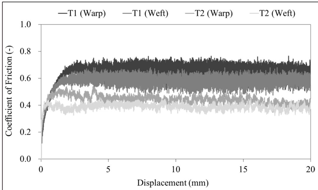
Figure 3-5 Friction coefficient curves measured with TL-201Ts
