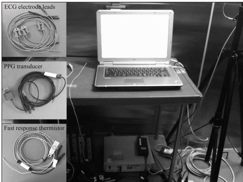
Figure 4-6 The MP 100 data acquisition system used for physiological measurement
