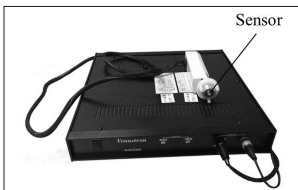
Figure 4-2 Venustron II used for compression property measurement
