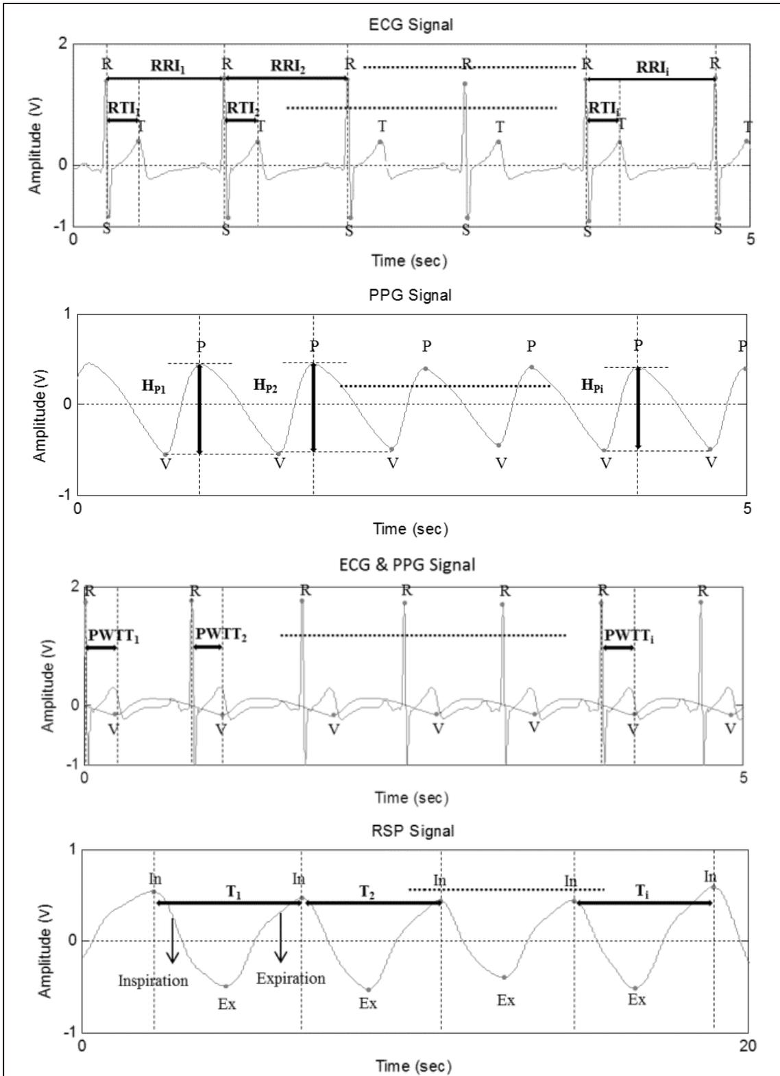
Figure 4-9 Signals used for physiological data acquisition
