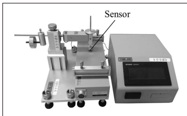
Figure 3-3 TL-201Ts used for surface property measurement
