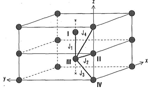
Fig. 2. Arrangement of Cu<sup>2+</sup> ions and exchange interactions between them.
