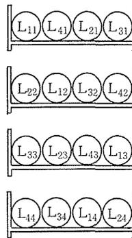
Fig.3 Another arrangement of the secondary windings in the bobbins
