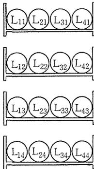
Fig.2 An arrangement of the secondary windings in the bobbins
