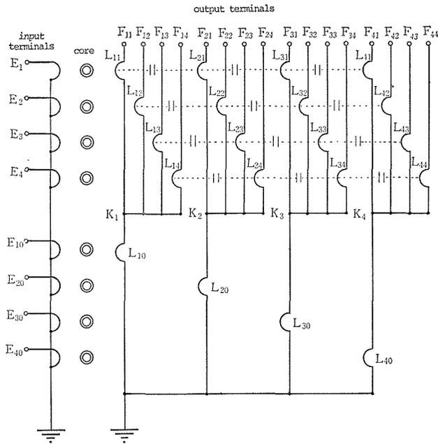
Fig.1 4 × 4 transformer assembly
