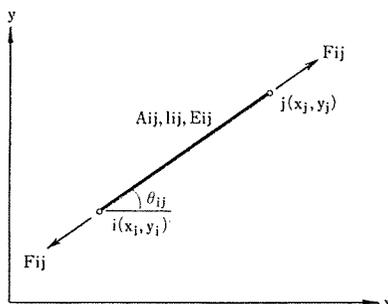
Fig. 1. A Member of a Truss.
