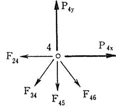
Fig. 5. Force Diagram at 4
