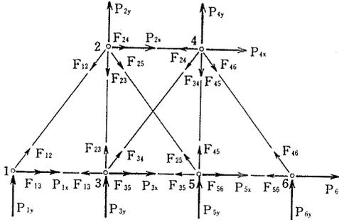
Fig. 3. Force Diagram at Each Joint
