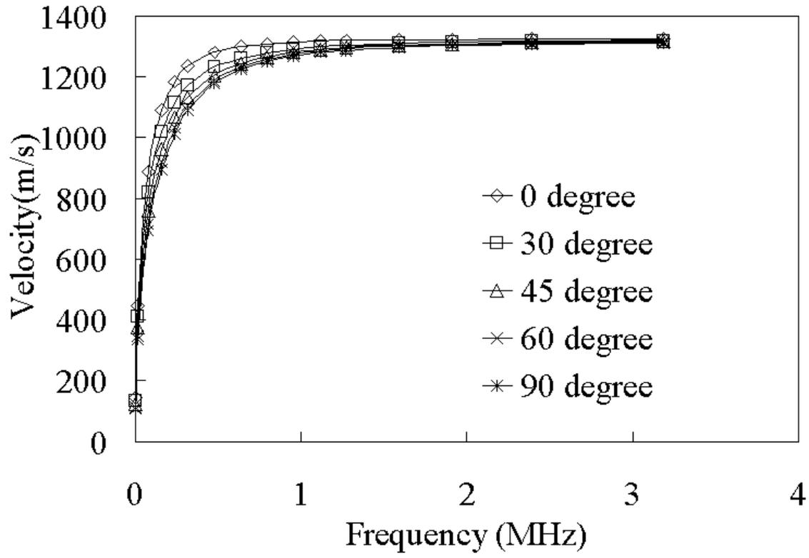
Figure 3 Velocity curves of  $A_0$  mode of 16-ply unidirectional laminated plate in different propagating directions.
