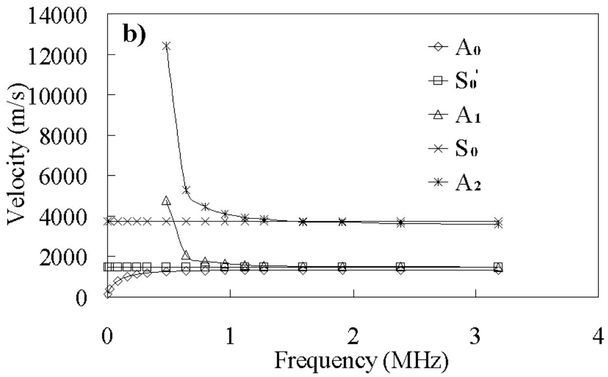
Figure 6 Influence of stacking sequence on dispersion curves along 0 degree direction of propagation.
