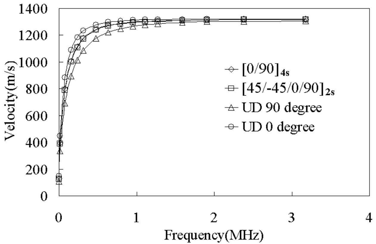
Figure 7 Velocity curves of A<sub>0</sub> mode of 16-ply laminated plate with different stacking sequences.
