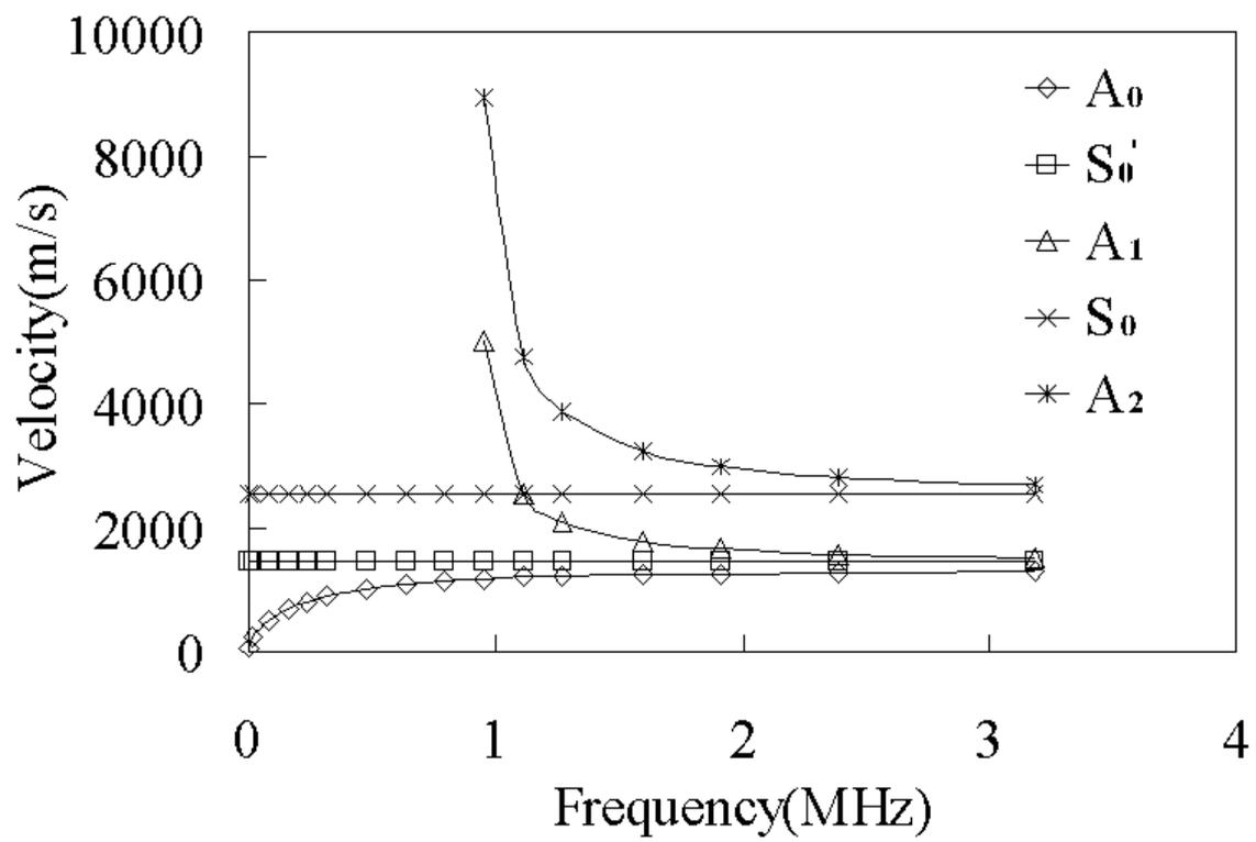
Figure 4 Dispersion curves of 8-ply unidirectional laminated plate in the direction perpendicular to fiber.
