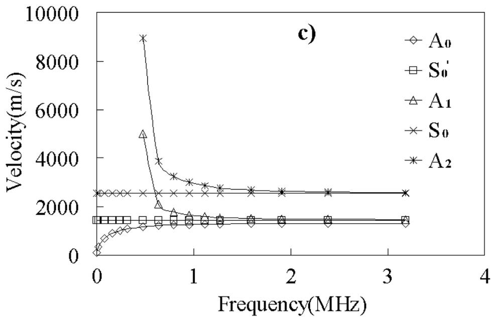
Figure 2 Dispersion curves of 16-ply unidirectional laminated plate.
