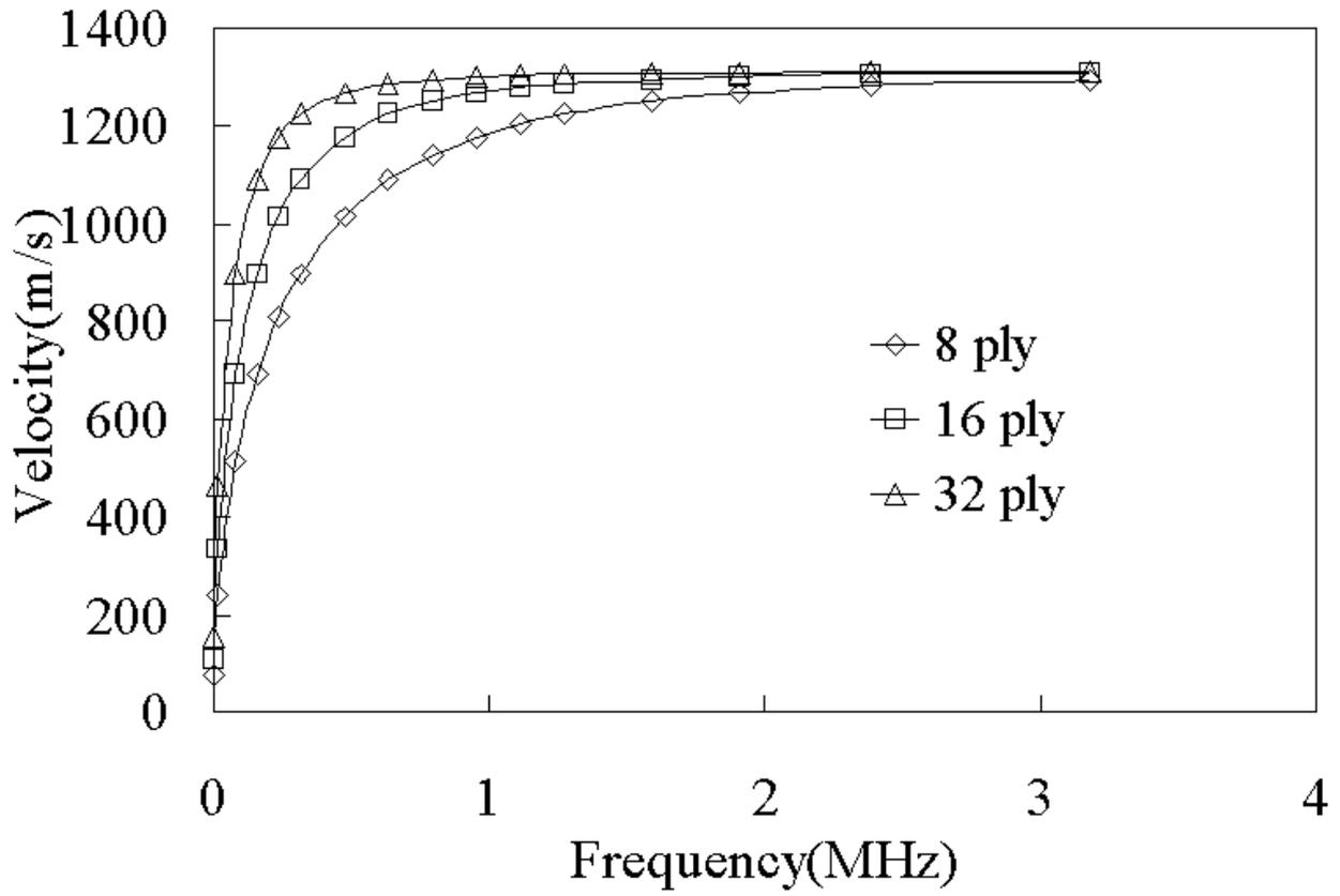
Figure 5 Velocity curves of  $A_0$  mode of unidirectional laminated plates in the direction perpendicular to fiber with different thicknesses.
