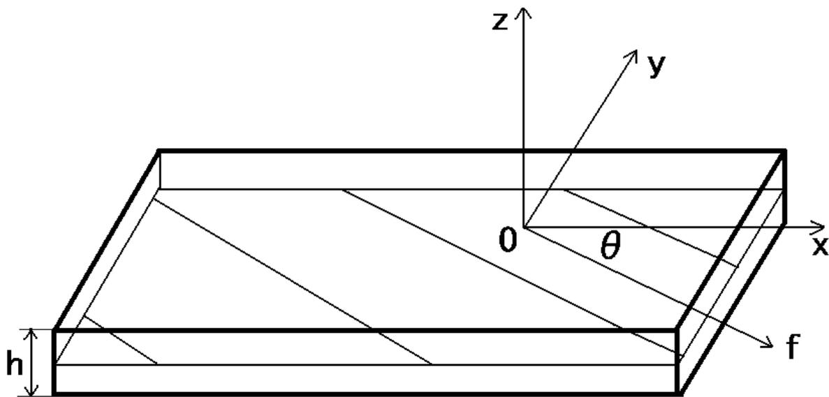
Figure 1 Coordinate axes of a laminated plate.
