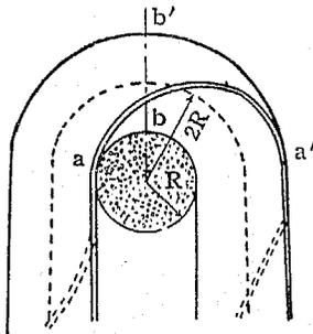
Fig 4. Diagram of the relaxation of fibers on the bending deformation of yarn.
