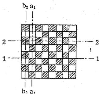
Fig 1. A plain fabric structural diagram
