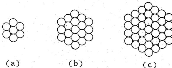
Fig 5. Ideal cross section of yarn.
