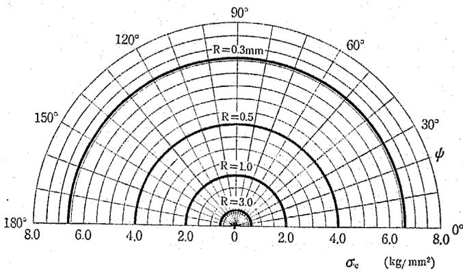
Fig 9. Diagram of the stress  $\sigma_c$  on the apparent central fiber
