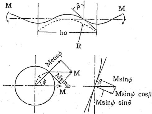
Fig 6. Moment diagram of the side fiber in bending yarn.
