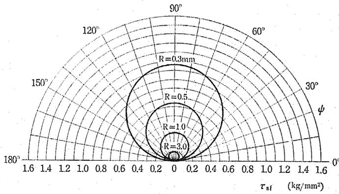
Fig 8. Diagram of the bending stress  $\sigma_{sf}$  and the torsional stress  $\tau_{sf}$  on the fill side fiber.
