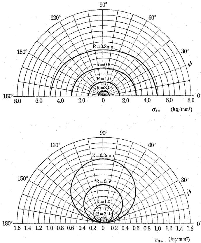
Fig 7. Diagram of the bending stress  $\sigma_{sw}$  and the torsional stress  $\tau_{sw}$  on the warp side fiber.
