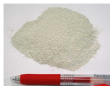
(c)多孔質ケイ酸カルシウム ( D_{50}=182\mu\text{m} )
