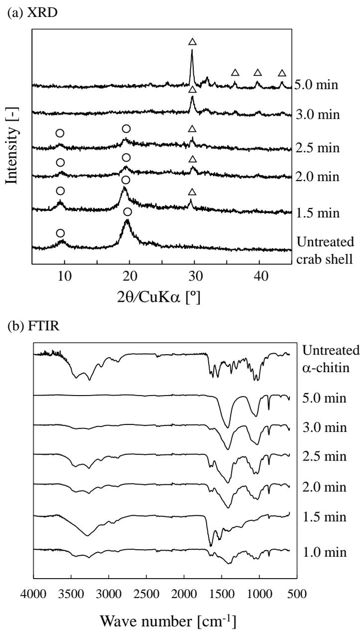
Fig. 3 Effects of supercritical water treatment at  $400^\circ\text{C}$  on the properties of crab shell: (a) XRD pattern ( $\circ$ :  $\alpha$ -chitin,  $\triangle$ :  $\text{CaCO}_3$ ) and (b) FTIR spectra.
