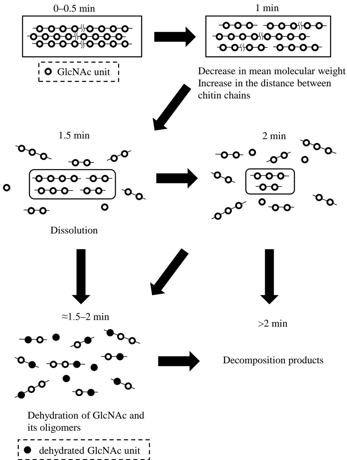
Fig. 7 Schematic of  $\alpha$ -chitin reaction in supercritical water.
