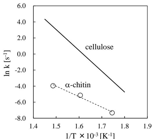
Fig. 6 Arrhenius plot overlay of first-order decomposition rate constants for the degradation of cellulose and  $\alpha$ -chitin.
