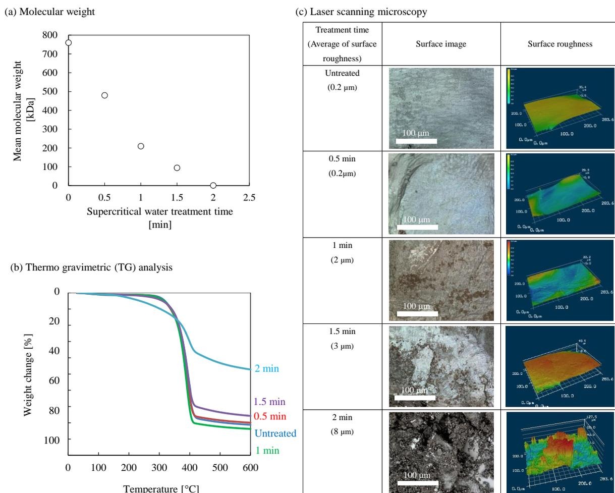
Fig. 5 Effects of supercritical water treatment at 400°C on the properties of pure  $\alpha$ -chitin: (a) mean molecular weight, (b) TG curves, and (c) surface roughness observed by laser scanning microscopy.
