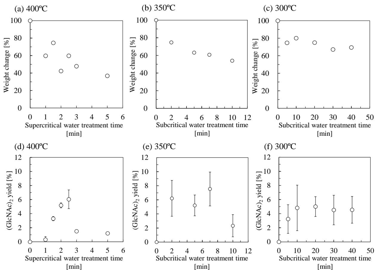
Fig. 1 Effect of sub- and supercritical water pretreatment time on weight change of crab shell and its enzymatic degradation (n = 3, bars indicate SEs).
