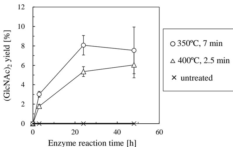
Fig. 2 Reaction time profile for enzymatic degradation of untreated, sub- and supercritical water treated crab shell (n = 3, bars indicate SEs).
