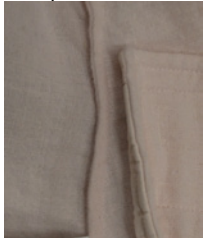
Figure 11. Example of low-quality piping seam finishing (C13)
