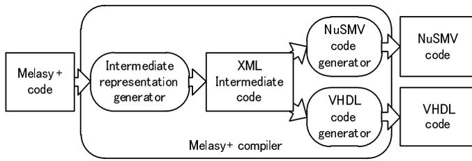
Fig. 1. Positioning of Melasy+ compiler and code generation
