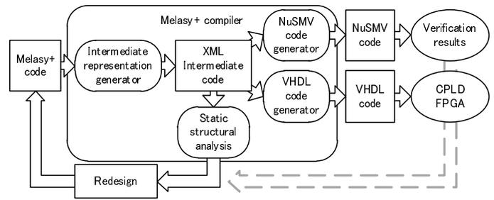
Fig. 2. Design cycle using generated codes or intermediate codes
