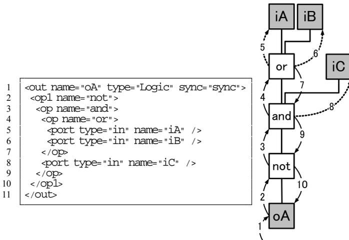
Fig. 4. Example of Node instance connection for output port definition
