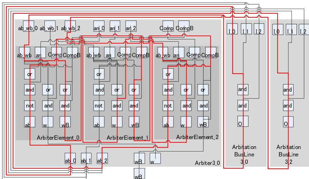
Fig. 7. Example of detection of asynchronous loop structure for Netlist
