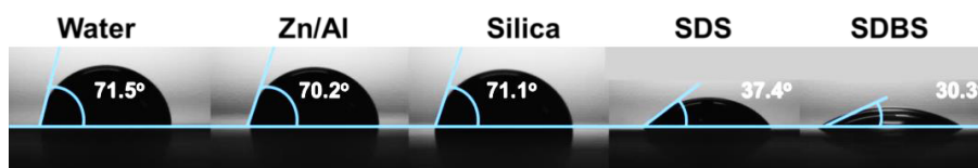
Figure 4-5. Contact angle of SWCNT inks and water on the PET substrate. Here Zn/Al, silica, SDS, and SDBS denote SWCNT inks dispersed with Zn/Al complex, silica, SDS, and SDBS, respectively.
