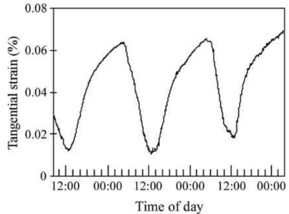
Fig. 4 Changes in tangential strain on the inner bark surface of a field-grown *C. japonica* tree at the end of July.
