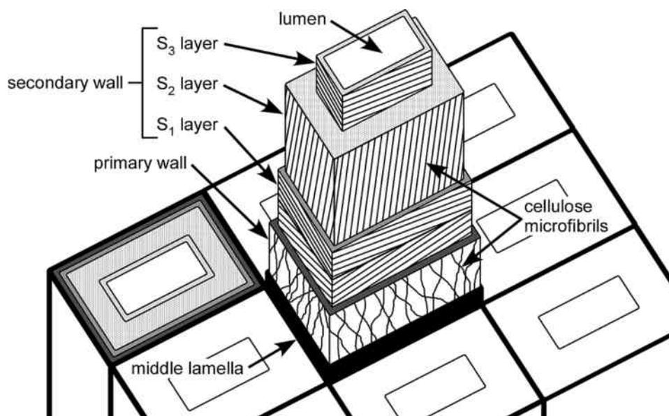
Fig. 1 A schematic model of the cell wall structure of a softwood tracheid.
