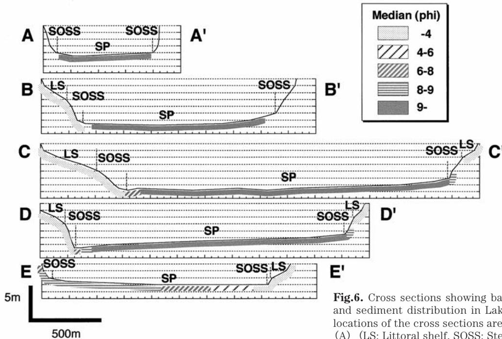
**Fig.6.** Cross sections showing basin topography and sediment distribution in Lake Kitaura. The locations of the cross sections are shown in Fig.4 (A) (LS: Littoral shelf, SOSS: Stepoff and sublacustrine slope, SP: Sublacustrine plain)
