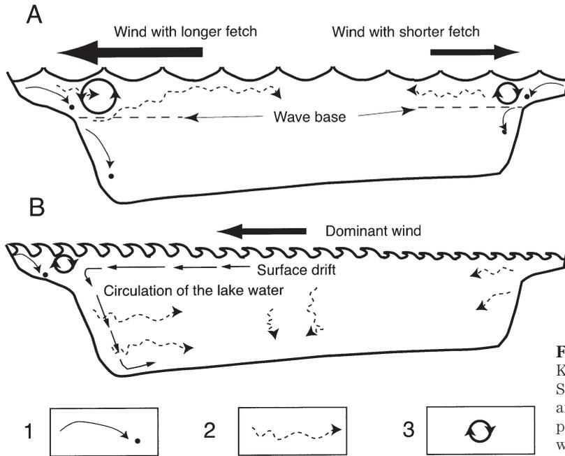
**Fig.8.** A model of sedimentary processes in Lake Kitaura predominantly affected by wind. A: Storm setting. B: Fair weather setting. 1: Erosion and transportation of sandy particles. 2: Transportation of clayey particles. 3: Influence of the wave action
