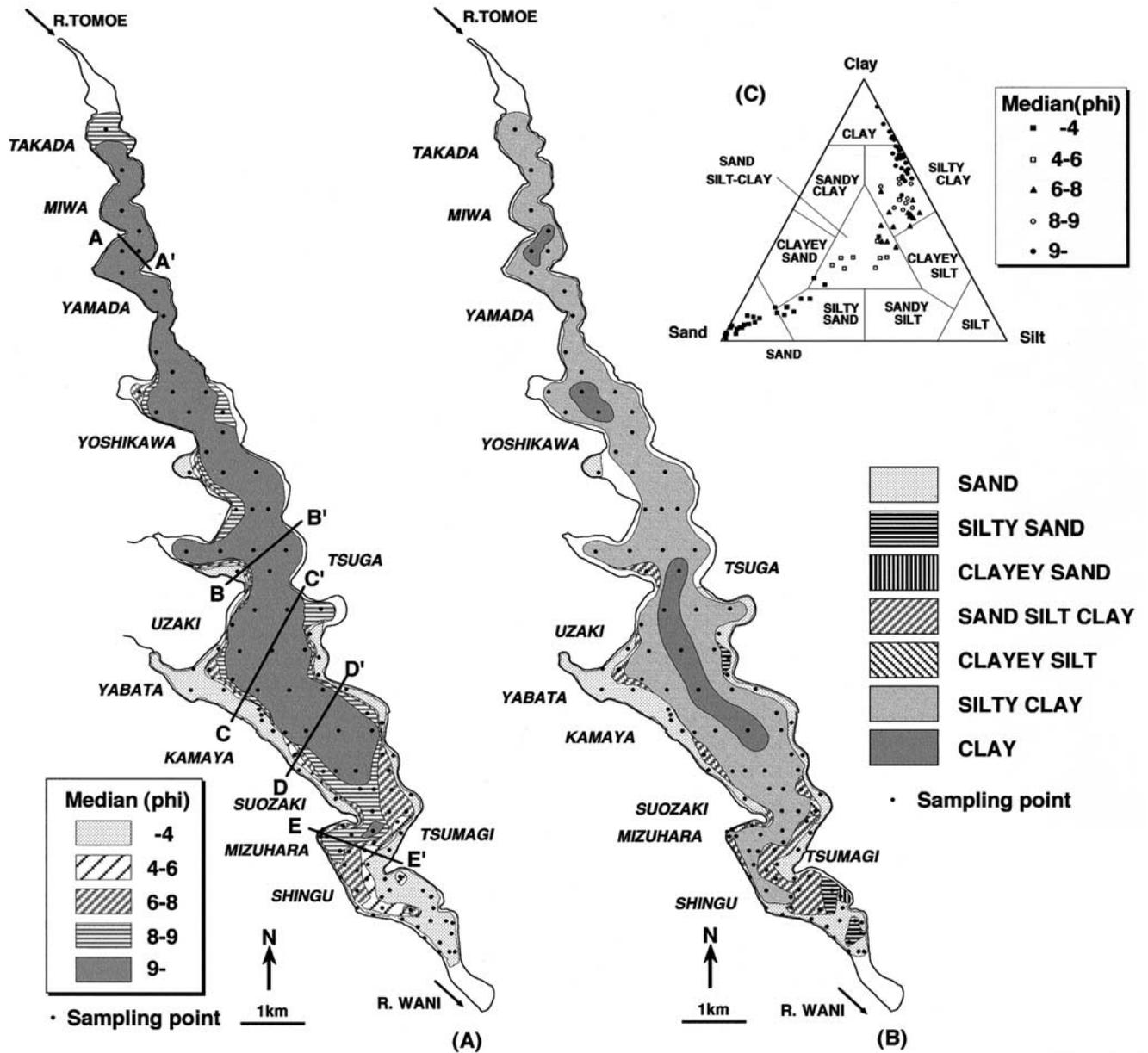
Fig.5. Grain size distribution of surficial sediments in Lake Kitaura. (A) Median diameter distribution shown in phi scale. (B) Distribution of sediments based on the nomenclature shown in diagram C. (C) Plots on a ternary diagram based on sand, silt and clay ratios (Shepard, 1954)
