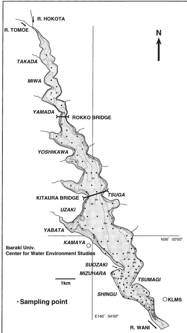
**Fig. 4.** Bathymetry of Lake Kitaura showing contours at 1m interval and sampling points of bottom surface sediments. KLMS: Kashima Local Meteorological Station
