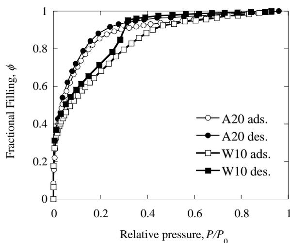
Figure 1. Adsorption isotherms of  $\text{CHCl}_3$  on ACF samples at 298K.
