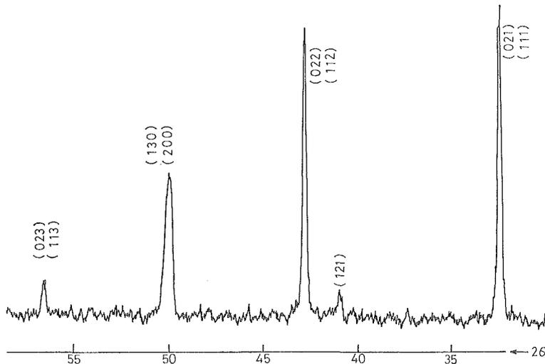
Fig. 1 : The diffraction pattern in  $\text{MnAs}_{0.97}\text{P}_{0.03}$  at room temperature.
