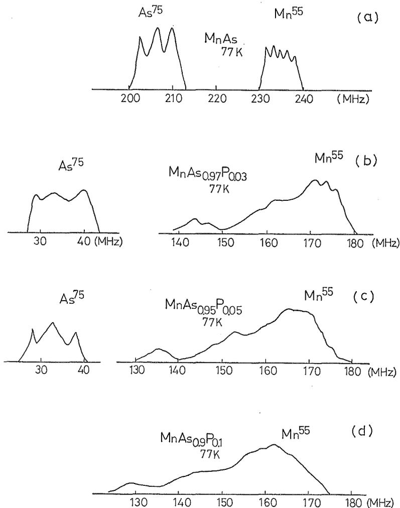
Fig. 3 : The  $Mn^{55}$  and  $As^{75}$  NMR spectra observed by spin echo method at 77 K.
