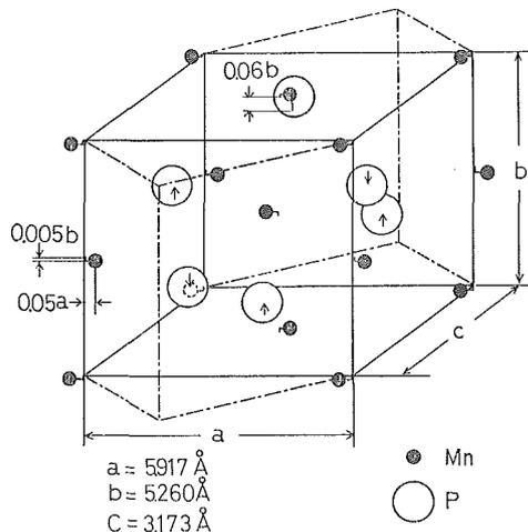
Fig. 2 : Orthorhombic B31 structure of MnP showing its relationship to hexagonal  $\text{B8}_1$  structure.
