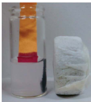
Fig. 4 The behaviour of Co@SiO 2 exposed to a magnet (right-side) after immersion in 1 M HCl. Particles in the sample bottle were attracted to the magnet. The photograph also shows that the color of the pH indicator paper turned from yellow to red in the acid solution.
