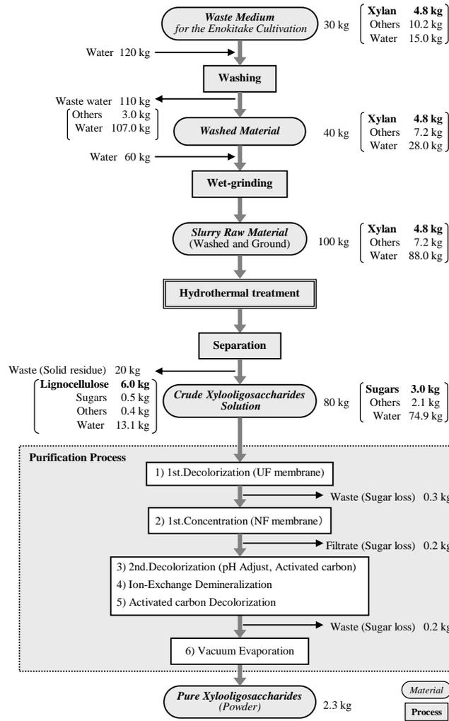
Fig. 4. Material balance of xylooligosaccharide production process with hydrothermal treatment for the waste medium.
