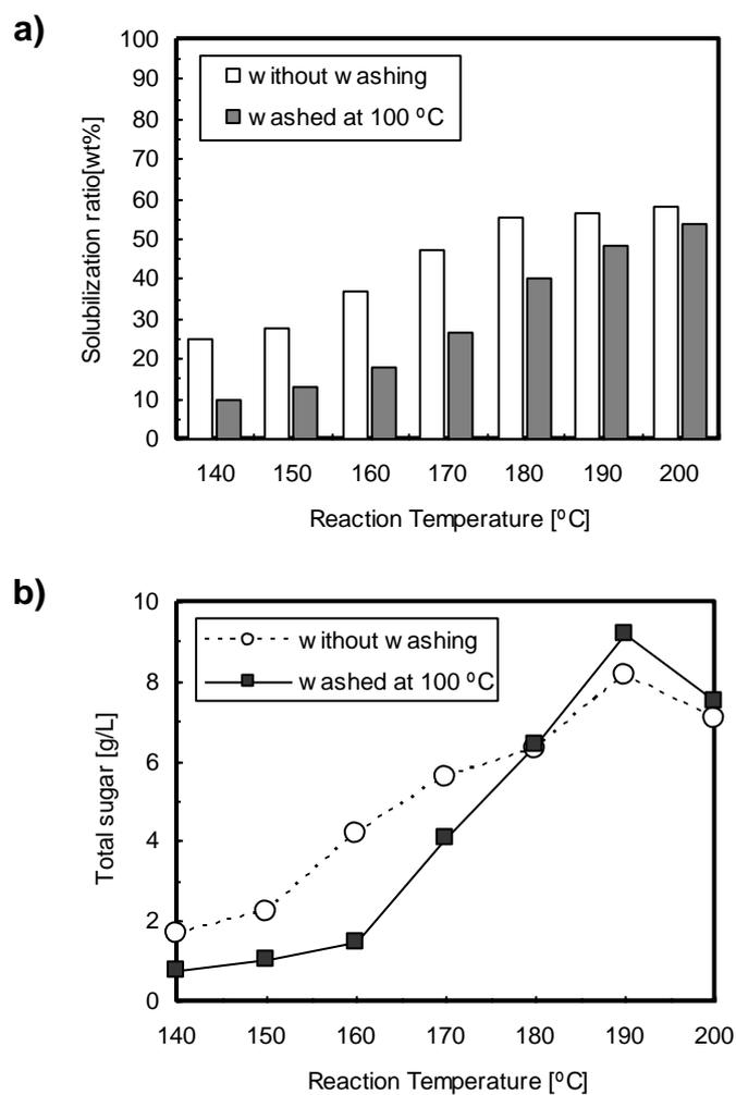
Fig. 1. Washing effects on a) solubility and b) total sugar for the hydrothermal treatment. The hydrothermal treatment were tested for waste medium without washing (white, circle) and waste medium washed at 100°C (black, square).
