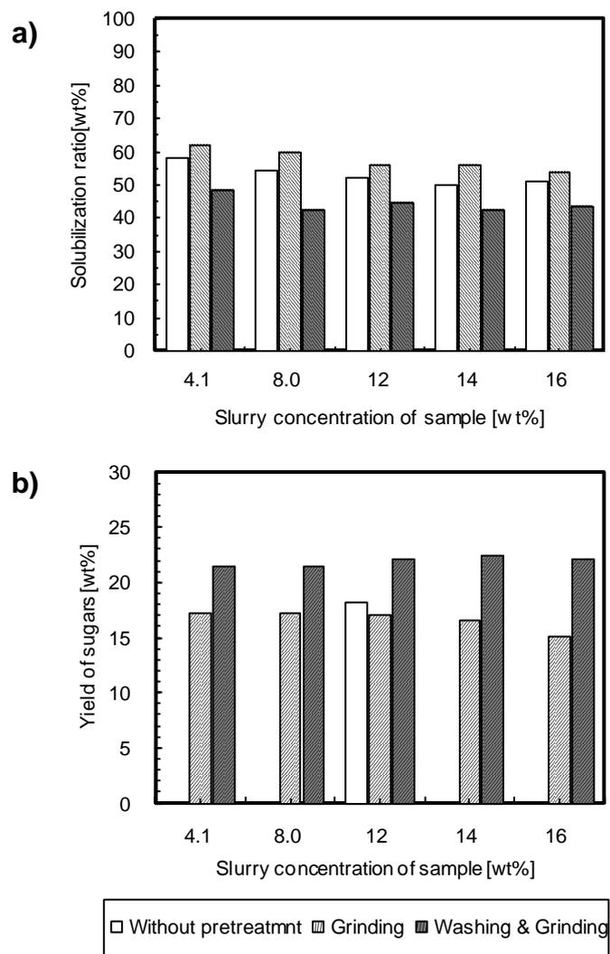
Fig.3 Effects of slurry concentration on a) solubility and b) yield of sugars for the hydrothermal treatment of the waste medium with or without washing and/or grinding.
