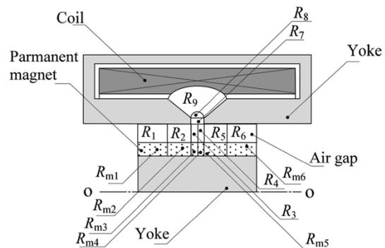
Fig. 2. Permeance model in the moving magnet-type LA.
