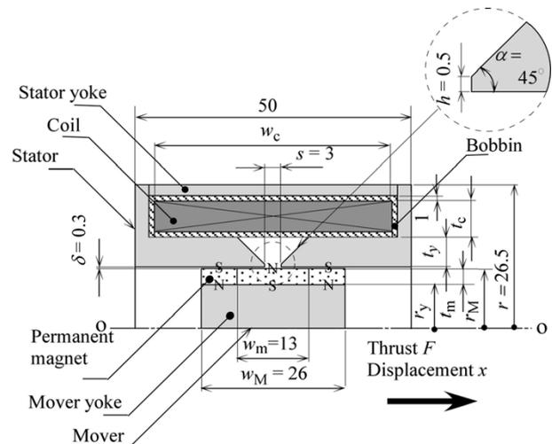
Fig. 1. Basic structure of a cylindrical moving magnet-type LA (unit: millimeters).
