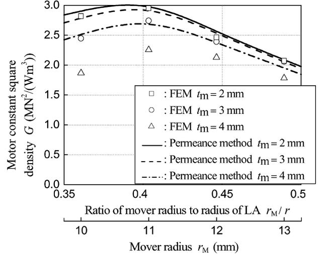
Fig. 4. Motor constant square density dependence with the mover radius as the parameter of permanent magnet thickness in both permeance method and FEM ( $NI = 500$  A).
