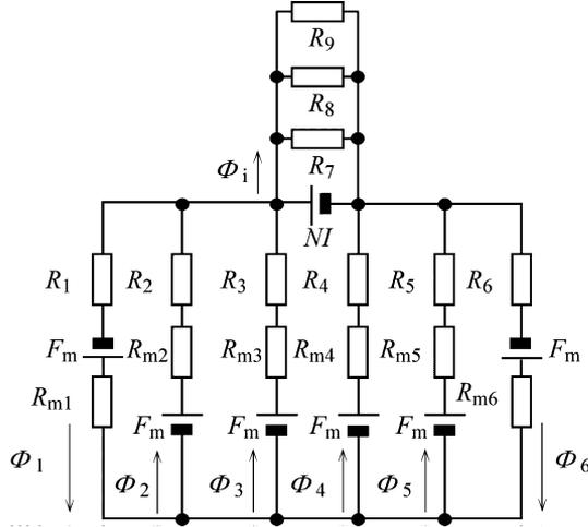
Fig. 3. Magnetic equivalent circuit of the moving magnet-type LA.
