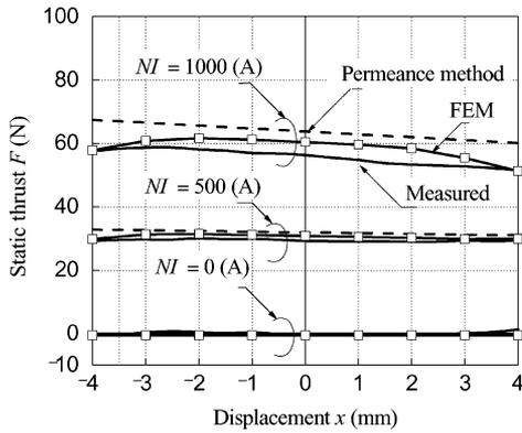
Fig. 6. Static thrust versus displacement characteristics of the moving magnet type LA.
