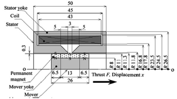
Fig. 5. Basic structure of the moving magnet-type prototype LA (unit: millimeters).
