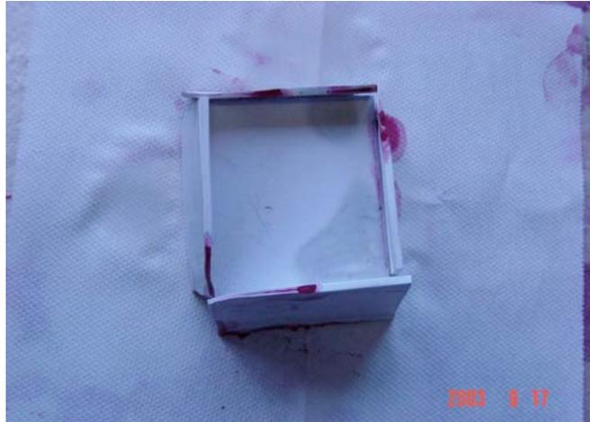
Fig. 5 Picture of cut and color checked sample
