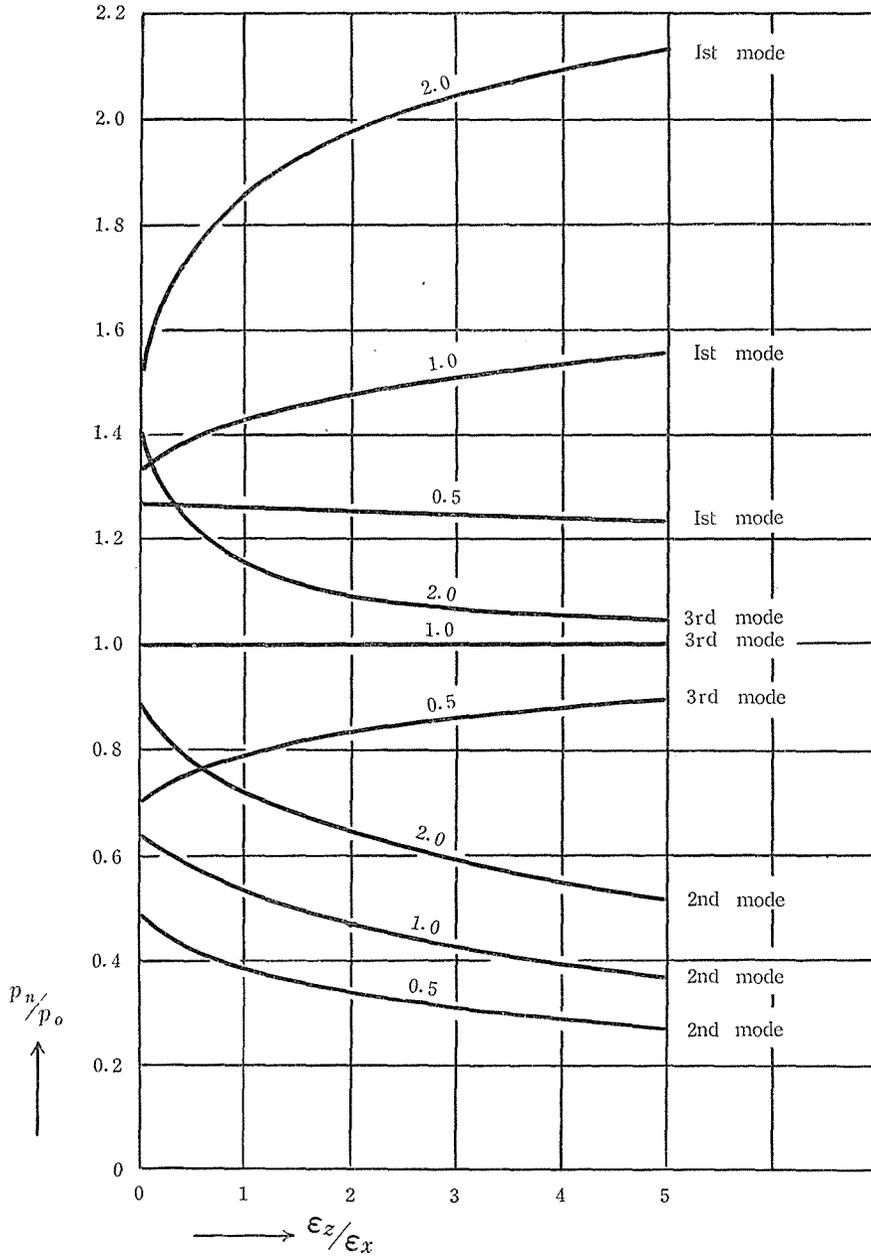
it is seen that computations of the natural frequencies of such a beam, in which the effects of the eccentricity are neglected, are apt to lead erroneous results.
