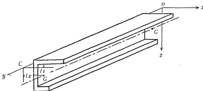
Fig. 1. Type of Beams in which Centroidal Axis is not Collinear with Shear-Center Axis.
