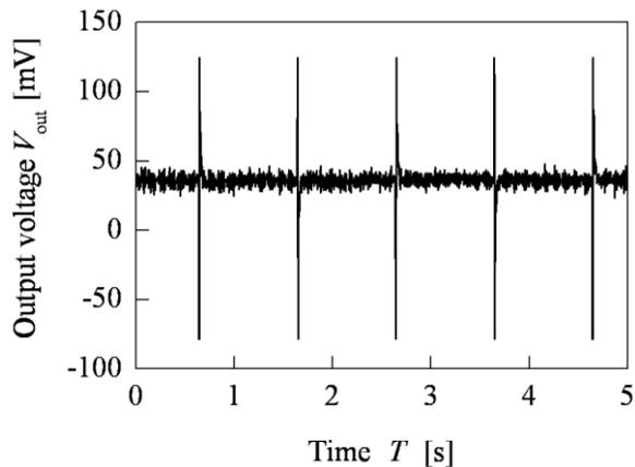
Figure 7. An example of the observing magnetic field from the watch measured with IG under the condition 7.
