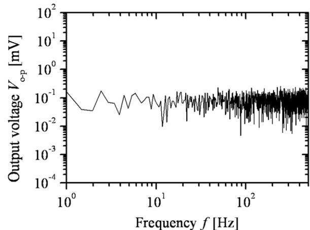
Figure 4. FFT analysis result of measured output voltage of the converter with a dummy load of  $150 \Omega$ .
