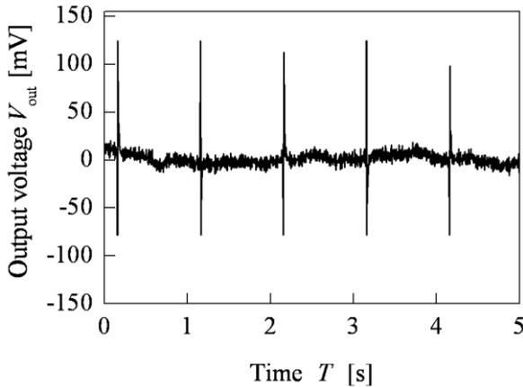
Figure 6. An example of the observing magnetic field from the watch measured with IG under the condition 6.
