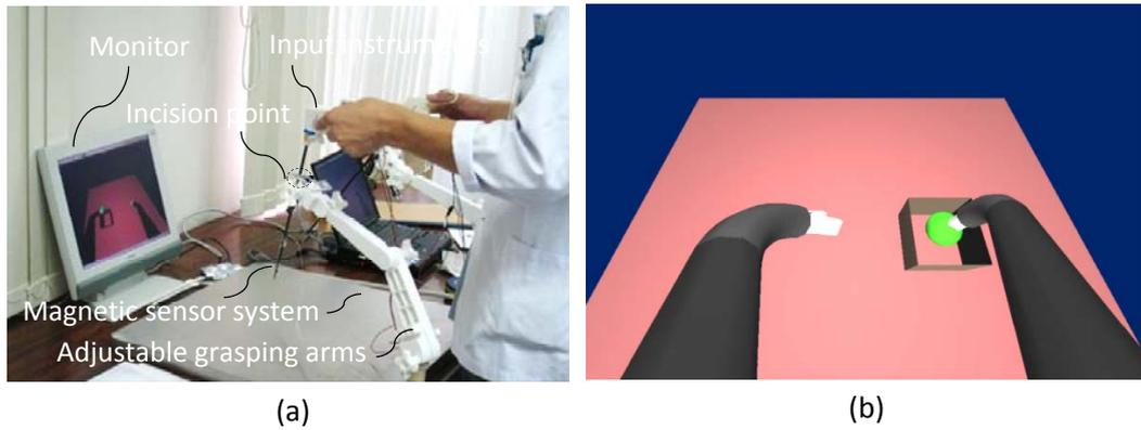
Fig. 4 Simulation experiment. (a) Manipulation on the master side. (b) Virtual image on the slave side.
