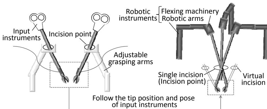
Fig. 2 Reflection of the instruments position and pose
