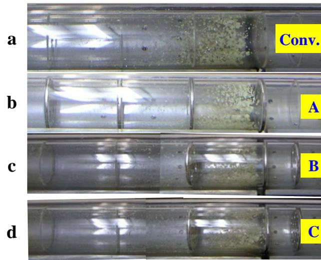
Fig. 3. Some representative results of purification of BCP under various purifying conditions; (a) a conventional method without introducing baffles, (b) introducing baffles only in  $T_h$  region, (c) introducing baffles with four orifices in both of  $T_h$  and  $T_l$  regions, and (d) the same setting with (c) except the number of orifices of baffles (16 orifices).
