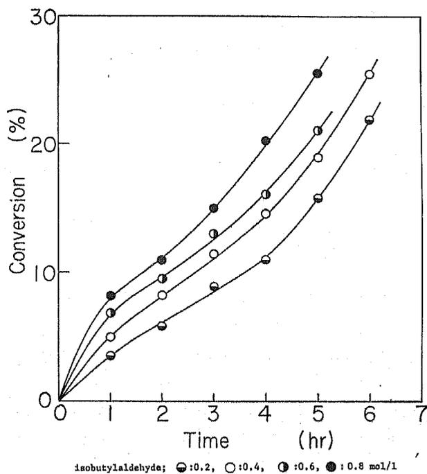
Fig.3. Effect of isobutylaldehyde concentration (methacrylic acid : 2.0 mol/l, 55°C).
