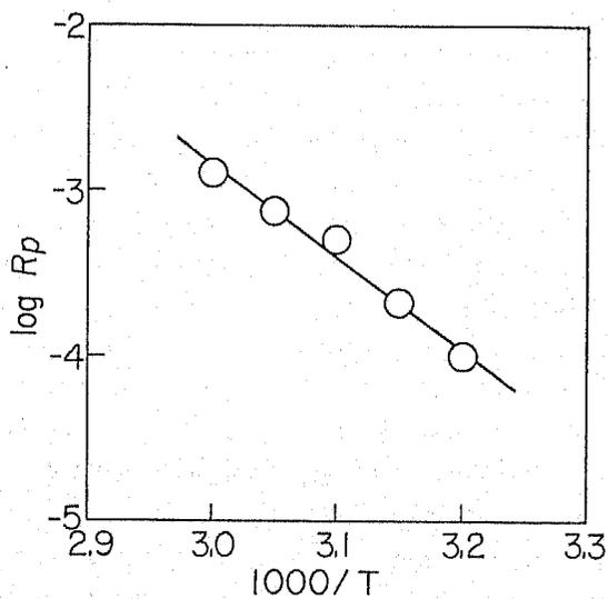
Fig. 2. ARRHENIUS plot of the rate of polymerization (methacrylic acid : 2.0 mol/l, isobutylaldehyde : 0.2 mol/l).
