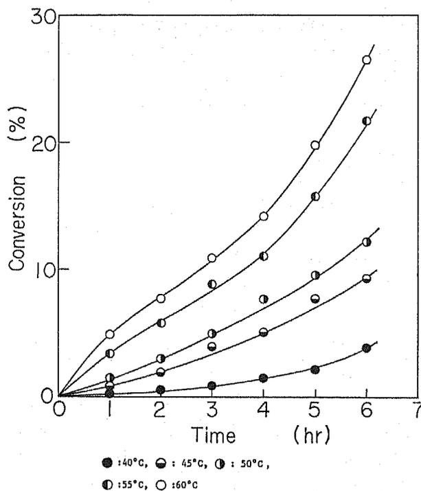
Fig. 1. Effect of temperature (methacrylic acid : 2.0 mol/l, isobutylaldehyde : 0.2 mol/l).
