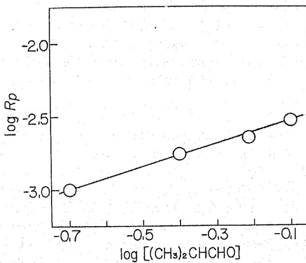
Fig.4. Relation between the rate of polymerization and the concentration of isobutylaldehyde (methacrylic acid : 2.0 mol/l, 55°C).
