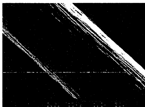
Fig.1 SEM image for the precursor fiber of TiO 2 +HEC. ([TiO 2 ]/[HEC]=6)
