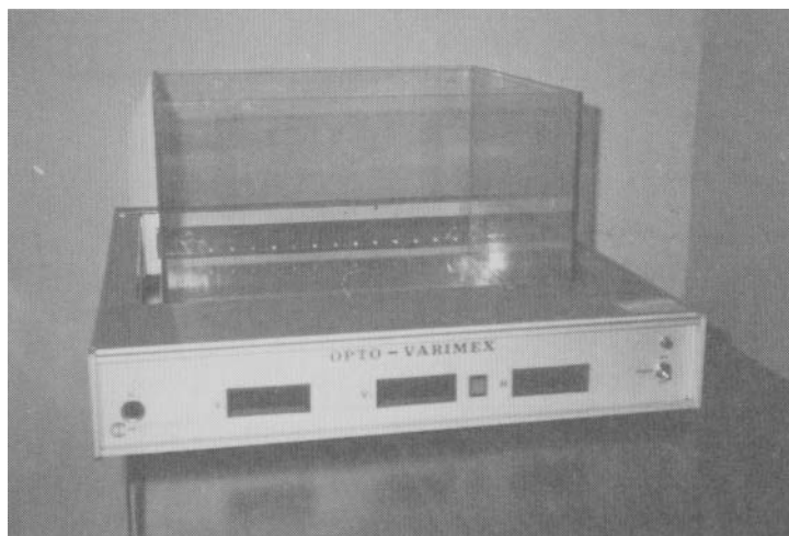
Fig. 3. Open-field apparatus. Size of the field is 40cm square. Each side has infrared sensor at 2.5cm interval and the locomotion was recorded by X-Y plotter. At the test 80cm high cover was applied on top to avoid an escape.
