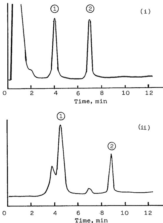
Fig. 1 GLC (i) and LC (ii) spectra of standard naringin and naringenin
