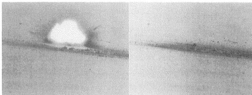
Figure 15 ACE explosion on hard snow at snow surface
