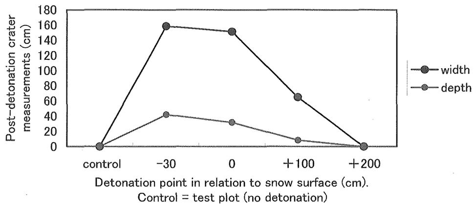
Figure 18 Crater size in relation to ACE detonation height (Craters range from 0-160 in width and up to 50 cm in depth)
