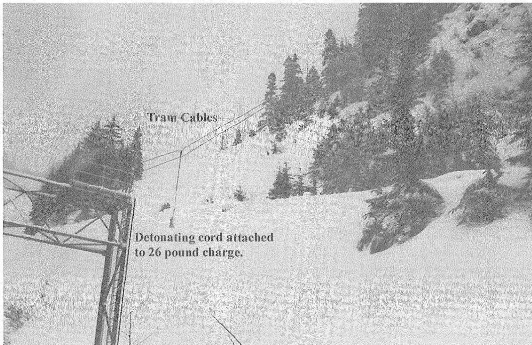
Figure 11 Bomb tram (raising type) shown with 12kg ANFO charge
