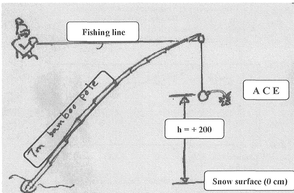
Figure 17 Improvised ACE aerial detonation technique
