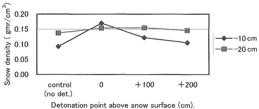
Figure 20 ACE post-detonation density change (in snow surrounding crater)
