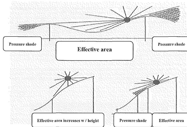
Figure 1 Explosion effective zone and shadow area
