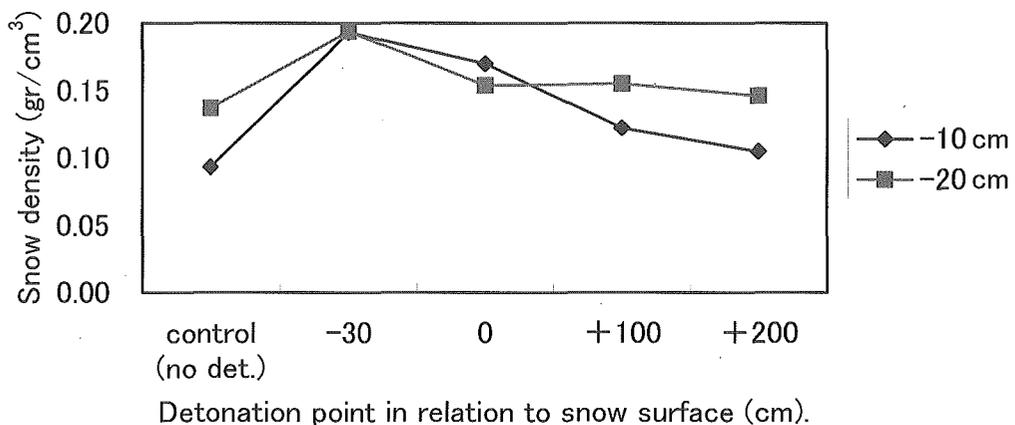
Figure 19 ACE post-detonation density change (in snow surrounding crater)
