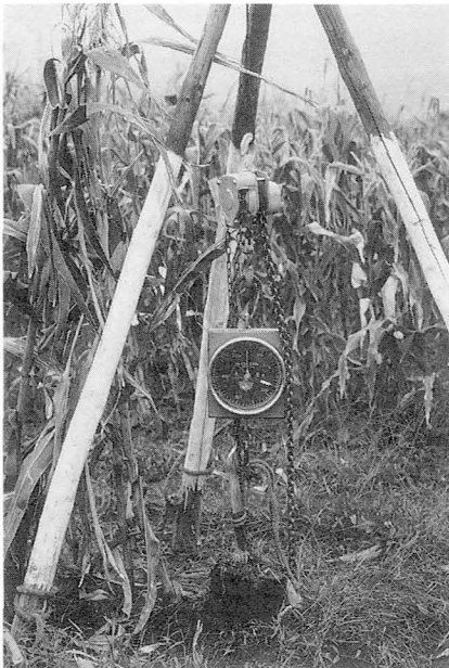
Fig. 4-6. Equipment for measurement of root-pulling resistance.
