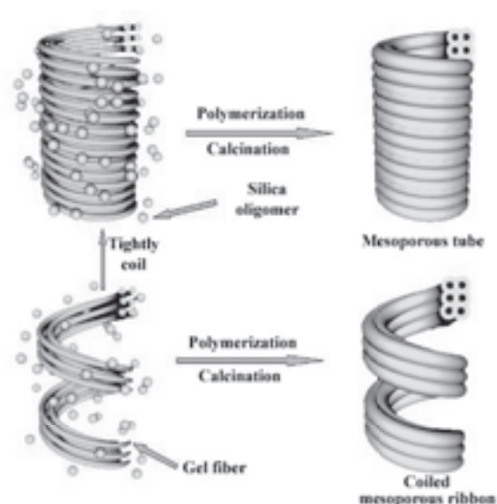
Fig. 6 Schematic representation of formation of coiled mesoporous silica nanoribbon and nanotube.
