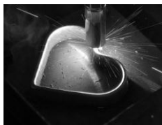
Photo.1.5 The latest free-design modeling technology by arc welding ; Metal 3D Print 24-1~3)
