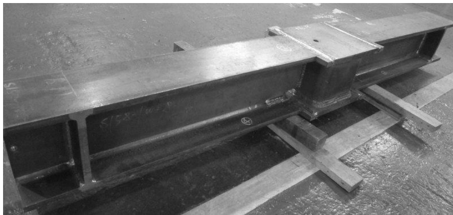
Photo 2.5 Appearance of the full-size beam-to-column test assembly
