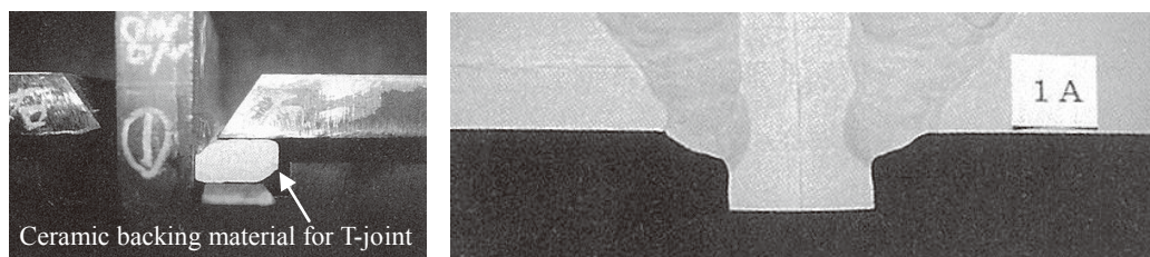
Photo 1.9 Ceramic backing material for T-joint and cross section shape of weld joint applying it 41-1)
