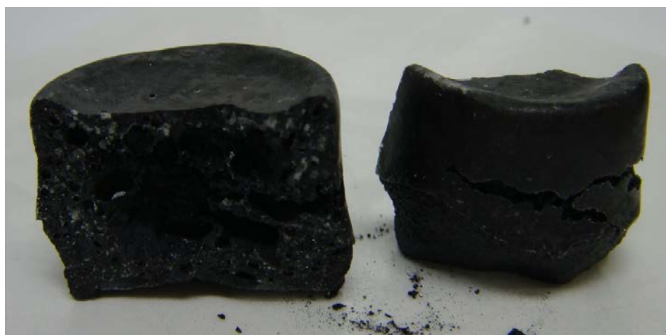
Fig.2.13 Digital photograph of product of LiCoO 2 crystals and NaCl flux.
