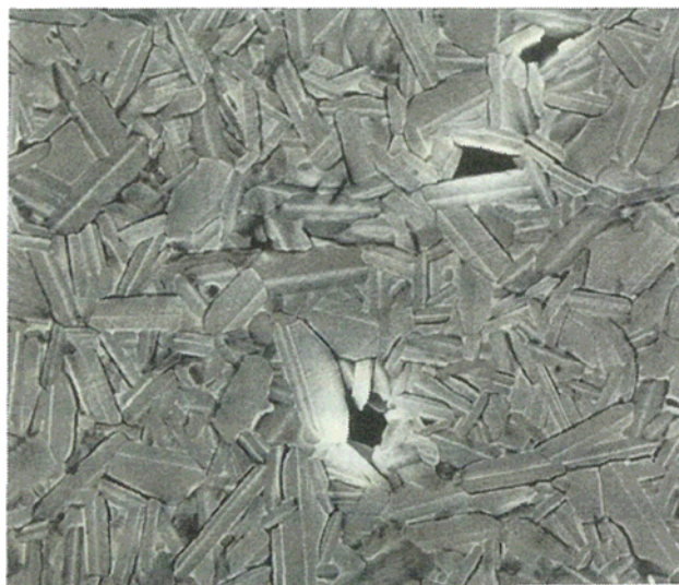
Fig. 1-3 Microstructures of SiC added Al 2 O 3 10) .
