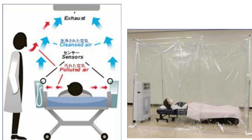
Figure 1-6 A ventilation system
