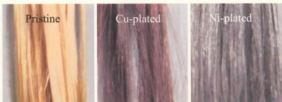
Fig. 4.3 Photographs of pristine and metal plated PBO fibers.
