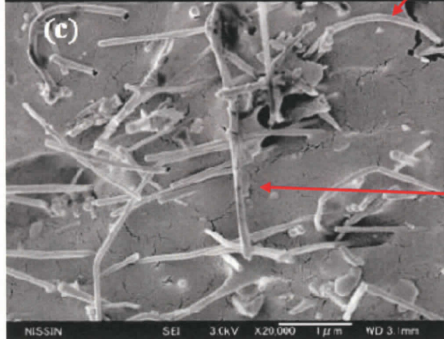
図 4.3 3 wt% MWCNT-A/FKM の引張破断面図(標準 CNT) SEM micrographs of MWCNT-1 raw materials Fig.3 (a) ×200, 3 wt% MWCNT-1/FKM composite Fig.3 (b) ×5k, and zoom in Fig.3 (c) ×20k
