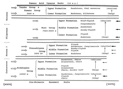
Fig. 3. Schematic illustration of the development of the Shimanto geosyncline in the Kii Peninsula. Arrow indicates a direction of sediment supply.
