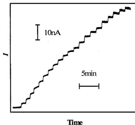
Fig. 2 Typical current-time response curve of the tyrosinase, NG-MTP-Au electrode on stepwise additions of catechol in 50 mM  $\text{Et}_4\text{NClO}_4\text{-AN}$  solution at  $-0.70$  V vs.  $\text{Ag}/\text{Ag}^+$ .
