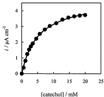
Fig. 3 Calibration plot of the tyrosinase, NG-MTP-Au electrode for catechol in 50 mM  $\text{Et}_4\text{NClO}_4\text{-AN}$  solution at  $-0.70$  V vs.  $\text{Ag}/\text{Ag}^+$ .
