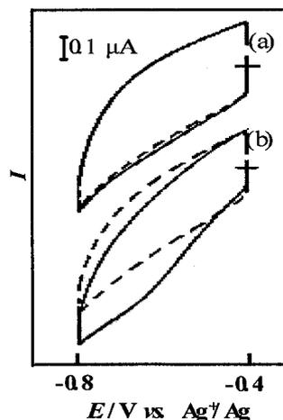
Fig. 1 Cyclic voltammograms of catechol in 50 mM  $\text{Et}_4\text{NClO}_4$ -AN solution at (a) Au and (b) the tyrosinase, NG-MTP-Au electrode. Dotted and solid lines were for blank and 30 mM sample solutions, respectively. Scan rate was 0.100 V/s.
