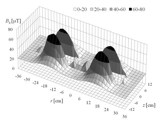
Fig. 7 Measured magnetic flux density in the axial direction when both modules were placed 10 cm apart in the radial direction.
