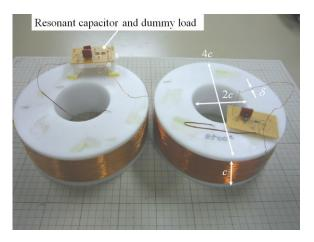
Fig. 1 Our developed energy harvesting modules.
