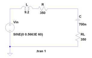
Fig. 2 A model of an energy harvesting module for a circuit simulator.
