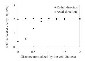
Fig. 6 Measured total harvested energy as a function of the distance normalized by the outer diameter of the coil.
