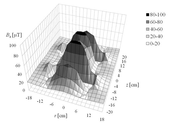
Fig. 8 Measured magnetic flux density in the axial direction when both modules were placed 10 cm apart in the axial direction.
