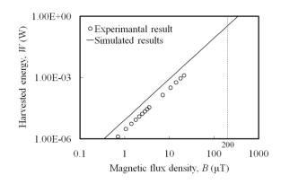
Fig. 4 Amplitude dependency of the modules. Plots represent measured results, and lines represent simulated results.
