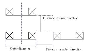
Fig. 5 Definition of the two distance parameters.
