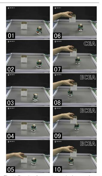
Fig. 11 Execution of cooperative sweeping between a human and a robot. The robot autonomously sweeps the top of the desk using a random spinning strategy and searches for the lifted object (1-5). It finds the lifted object (6) and approaches it (7), and sweeps the area under the object (8-10).
