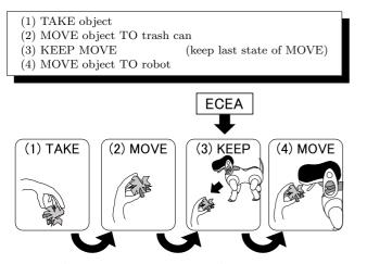
Fig. 18 ACS description with ECEA of garbage throwing. ECEA is used in (3). When the user pretends to throw the garbage to the trash can in (3), the robot approaches the user and take the garbage.
