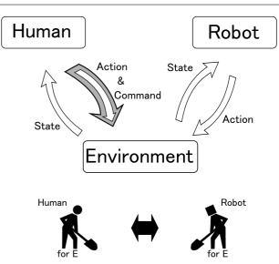
Fig. 2 CEA interaction model. Commands for robots are embedded in human actions. It has no direct command for robots. Users do not need to manipulate them and enables users to act for themselves and robots to make a decision based on the user's action.
