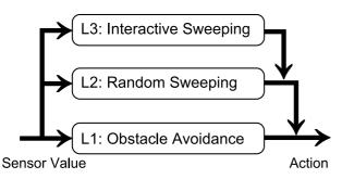
Fig. 10 Subsumption architecture. We designed three layers of robot behavior; the obstacle avoidance layer, the random sweeping layer, and interactive sweeping layer.
