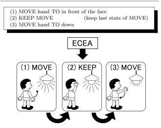
Fig. 17 ACS description with ECEA of room light dimming. ECEA is used in (2). Users send the command to dim the lights by screening their eyes from it with the hand.
