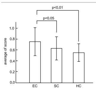
Fig. 16 Results of scores and differences. The scores are normalized by each participant's calculation ability. A score of 1.0 represents their calculation ability without controlling the robot. The Dunnett's multiple comparison test was used to statistically identify the significant differences in the scores from the control group (EC).
