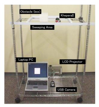
Fig. 13 Experimental system. The devices under the sweeping area include a laptop computer, a projector, and a USB camera with an infrared filter. The robot's location is obtained from the camera image that includes two infrared LED beams equipped on the robot. Based on the robot's location, it creates a projection image that includes small square cells and it is immediately colored when the robot enters the cell.
