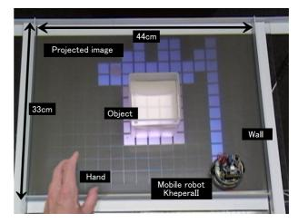
Fig. 6 Sweeping area. It has a flat surface to be swept, a wall enclosing the sweeping area, and a box placed in the center of it. Based on the robot's location, the projected image includes small square cells and it is immediately colored when the robot enters the cell. The colored cells represent the region swept by the robot.
