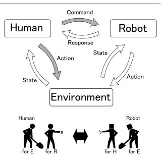
Fig. 1 DCM interaction model. A human directly sends commands to robots in order to control them. It includes methods using a remote control, voice commands, and gesture command.
