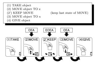
Fig. 9 ACS description of moving object using KEEP action. ECEA is used in (2'), and CEA is used in (2) and (3). The robot approaches the object when a user raises it (2). It sweeps the area under the object while the object is held above the area (2') and goes out of the area when the user lowers it (3).
