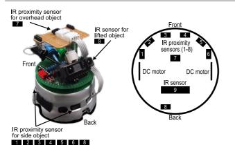
Fig. 7 KheperaII robot. The robot has eight infrared proximity and ambient light sensors with up to a 10 cm range (1-8). The sensors 1–6 and 8 directed to side, and the sensor 7 is directed upward. The sensor 7 is rearranged and the sensor 9 (SHARP GP2D12) with up to an 80 cm range for sensing a lifted object are added.
