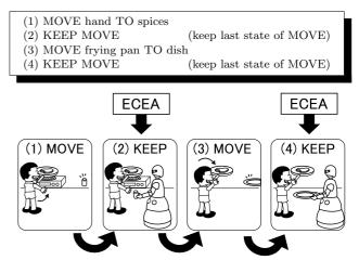
Fig. 19 ACS description with ECEA of a cooking task. ECEA is used in (2) and (4). When a user holds the hand during reaching the hand out for a spice bottle, a robot picks up the spice bottle and approaches to the user to pass it to her/him as shown in (2). When a user holds a frying pan during placing the food in a serving dish, the robot gives a dish to her/him as shown in (4).
