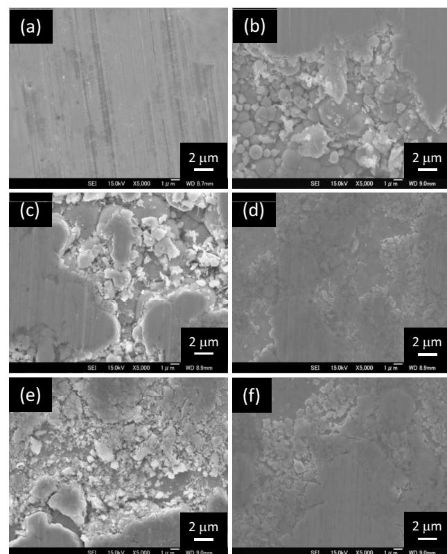
**Figure 10.** SEM images of worn surfaces of the high phosphorus-type films after the heat-treatment: (a) Ni-P alloy, (b) Ni-P alloy/Ilijin composite, (c) Ni-P alloy/VGCF composite, (d) Ni-P alloy/cut-VGCF composite, (e) Ni-P alloy/VGNF composite, and (f) Ni-P alloy/cut-VGNF composite film.
