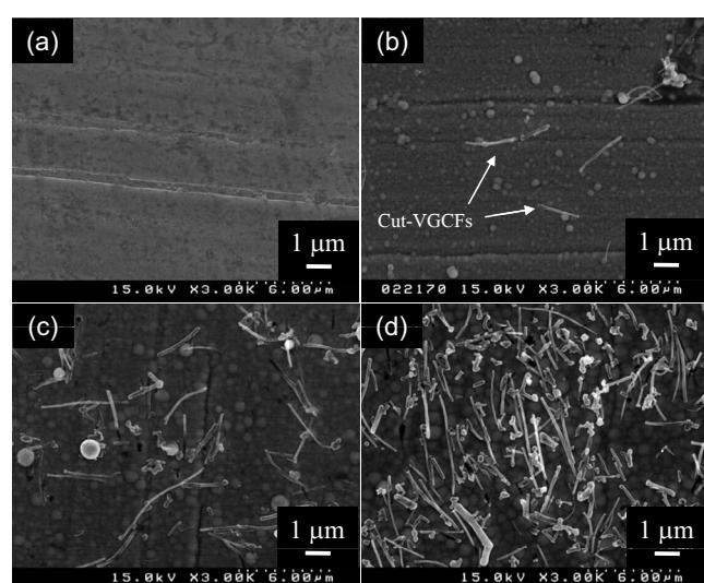
**Figure 1.** Surface SEM images showing the growth of electroless deposited Ni-P alloy/MWCNT composite films (a) before electroless deposition, (b) after 10 min, (c) after 30 min, and (d) after 60 min. The MWCNTs used are cut-VGCFs. The electroless plating bath used is the high phosphorus-type bath.
