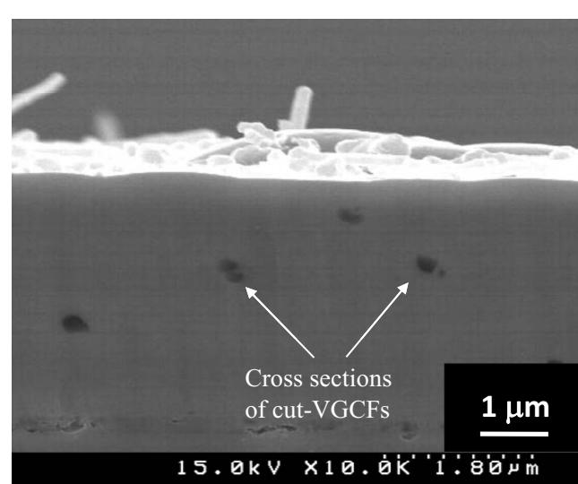
**Figure 2.** Cross-sectional SEM image of high phosphorus-type Ni-P alloy/cut-VGCF composite film. Film thickness is  $\sim 4$   $\mu\text{m}$ .
