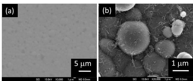
**Figure 5.** Surface SEM images of low phosphorus-type Ni-P alloy/Ilijin composite film. Film thickness is  $\sim 4 \mu\text{m}$ .
