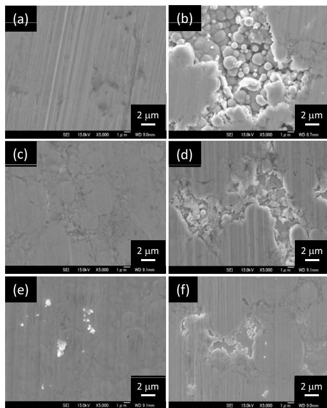
**Figure 9.** SEM images of worn surfaces of the high phosphorus-type films before heat-treatment: (a) Ni-P alloy, (b) Ni-P alloy/Ilijin composite, (c) Ni-P alloy/VGCF composite, (d) Ni-P alloy/cut-VGCF composite, (e) Ni-P alloy/VGNF composite, and (f) Ni-P alloy/cut-VGNF composite film.
