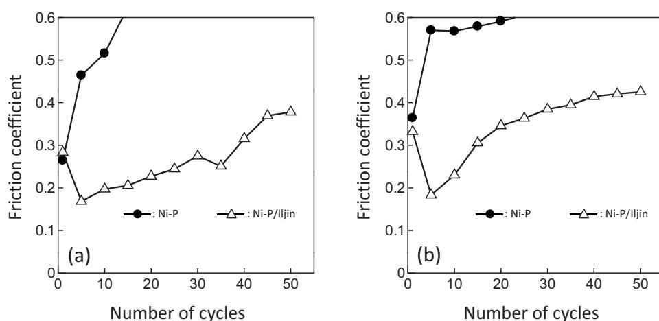
**Figure 12.** Friction coefficient as a function of number of cycles for the low phosphorus-type Ni-P alloy/Ijin composite film (a) before and (b) after heat-treatment.
