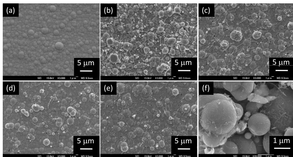
**Figure 4.** Surface SEM images of medium phosphorus-type Ni–P alloy/Various MWCNT composite films: (a) Ni–P alloy, (b) Ni–P alloy/VGCF composite, (c) Ni–P alloy/cut-VGCF composite, (d) Ni–P alloy/VGNF composite, (e) Ni–P alloy/cut-VGNF composite, and (f) Ni–P alloy/Iijin composite film. Film thickness of all films is ~4 μm.
