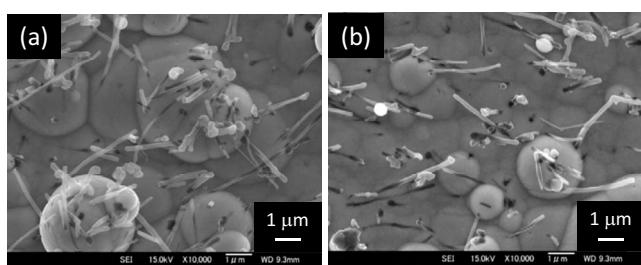
**Figure 6.** Surface SEM images of the medium phosphorus-type Ni-P alloy/cut-VGCF composite films (a) before and (b) after heat-treatment. Film thickness is  $\sim 4 \mu\text{m}$ . The heat-treatment condition was  $400^\circ\text{C}$  for 60 min.
