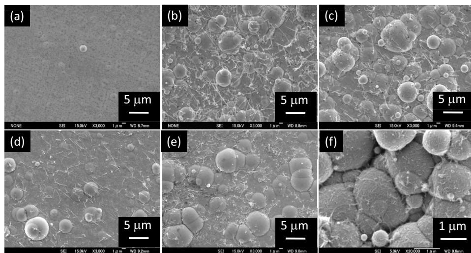
**Figure 3.** Surface SEM images of high phosphorus-type Ni–P alloy/Various MWCNT composite films: (a) Ni–P alloy, (b) Ni–P alloy/VGCF composite, (c) Ni–P alloy/cut-VGCF composite, (d) Ni–P alloy/VGNF composite, (e) Ni–P alloy/cut-VGNF composite, and (f) Ni–P alloy/Iijin composite film. Film thickness of all films is ~4 μm.
