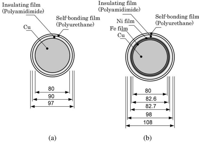
Fig. 2. Structures of COW and MPW (unit:  $\mu\text{m}$ ). (a) COW. (b) MPW.
