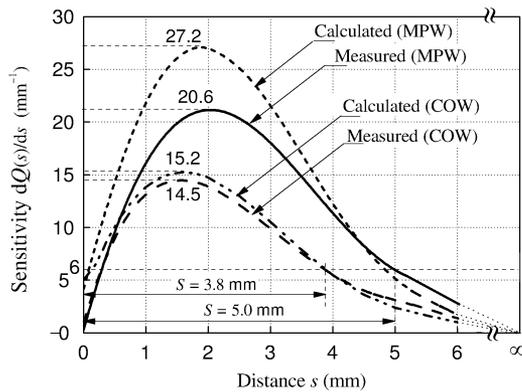
Fig. 7. Sensitivity versus distance characteristics (COW:  $f = 500$  kHz, MPW:  $f = 780$  kHz, measured with impedance analyzer HP 4192A).
