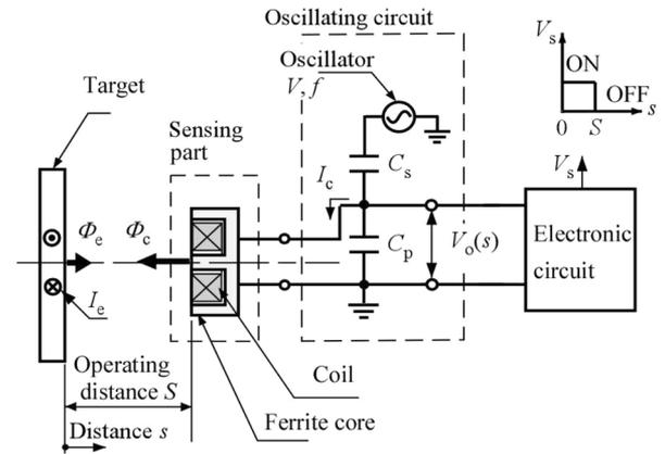
Fig. 1. Detection principle of inductive proximity sensor (coil:  $N = 100$  turns, ferrite core: Tomita Electric Co., Ltd. 2H6-PC-7  $\times$  2.1, target: cold rolling carbon steel sheet,  $1 \times 20 \times 20$  mm<sup>3</sup>).
