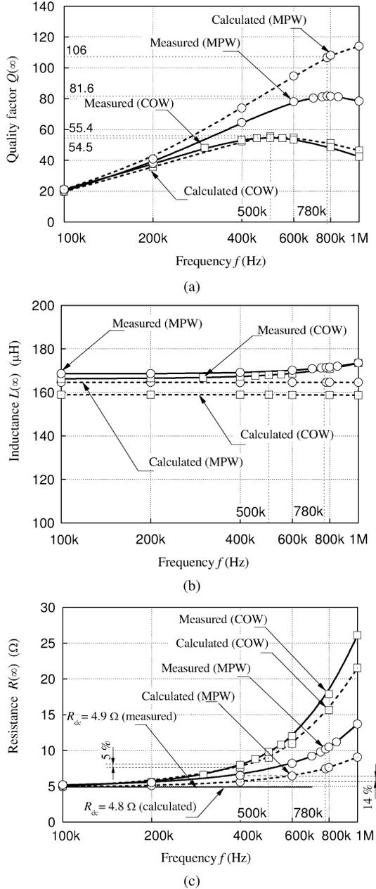
Fig. 4. Impedance versus frequency characteristics of COW and MPW sensing parts (measured with impedance analyzer HP 4192A). (a) Resistance. (b) Inductance. (c) Quality factor.
